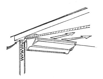
TV is designed to provide high capacity air inlets which are infinitely adjustable for both summer and winter.
