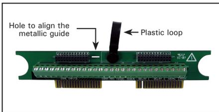
**!** *Before making the connections, pass the wires through an hermetic cable holders at the bottom of the enclosure.*
