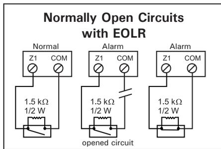
The following figures show different zone connection examples. Note that if you add an EOLR to a circuit, the resistor must be connected to the sensor that is furthest from the Agri-Alert system.
