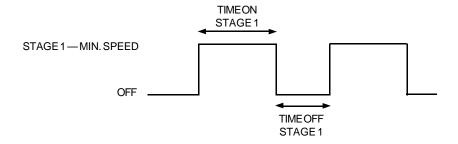
During TIME ON, the fans run at minimum speed. During TIME OFF, the fans do not run.
