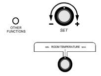
The reset erases the current minimum and maximum temperatures. From the moment the reset is completed, the controller begins to store in memory the new minimum and maximum temperatures measured by the probes.
