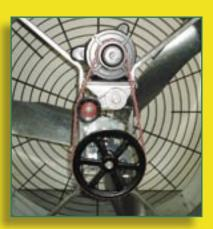
Motor mount and drive assembly utilize a rugged box frame design to increase motor life.
