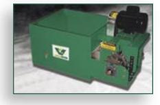
Two-line suspended drive hopper is used in breeder houses as an alternative configuration to the combination auxiliary/one-line drive hopper.
