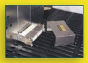
Dual roller return idler assembly at end of nest row provides adjustable belt tracking and brushes for belt cleaning. (Center belt idler assembly shown above; Side belt idler assembly shown below.)
