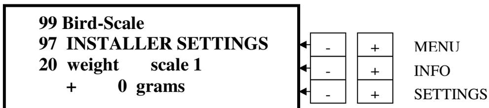
Press **INFO “+”** to go to **info 20**. Once the scale is calibrated, an actual weight will show in the value line. See **CALIBRATION Quick Sheet** for more details.
