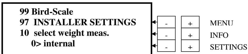
Press **INFO “+”** to go to **info 10**. This is preset to **Internal** for use with a single BE-SSC-101 installation. If a multiple BE-SSC-101 installation is used, then press the **SETTINGS “+”** button to change to **External**.
