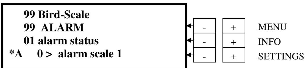
If the system goes into a state of alarm, you'll see the top info **“99 BE-SSC-101 Bird-Scale”** and at the bottom info an **“\*A”**, flashing off & on. There will be an alarm message in **info 0> - e.g. alarm scale 1**
