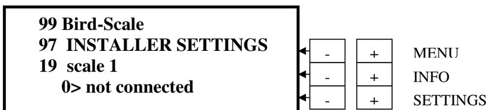
Press **INFO “+”** to go to **info 19**. To connect the scale, press **SETTINGS “+”** to get **1> connected**.
