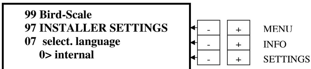
Press **INFO “+”** to go to **info 07**. This is preset to **Internal** for use with a single BE-SSC-101 installation. If a multiple BE-SSC-101 installation is used, then press the **SETTINGS “+”** button to change to **External**.
