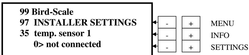
Press **INFO “+”** to go to **info 35**. If a temp sensor is attached, press **SETTINGS “+”** to get **1> connected**.
