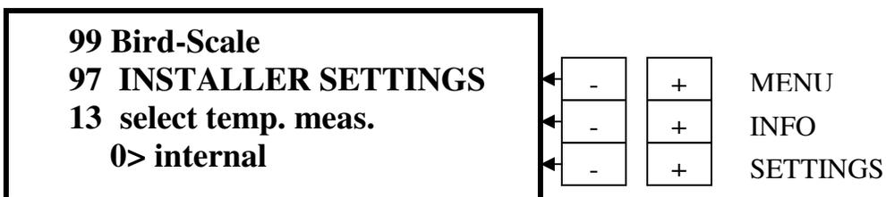
Press **INFO “+”** to go to **info 13**. This is preset to **Internal** for use with a single BE-SSC-101 installation. If a multiple BE-SSC-101 installation is used, then press the **SETTINGS “+”** button to change to **External**.
