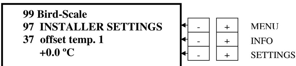
Press **INFO “+”** to go to **info 37**. You can adjust the temperature sensor by pressing **SETTINGS “+ or -”** or if more than one temperature sensor is activated, repeat the above steps for **Infos 38 – 46**. **Normally no action is required here.**
