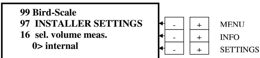
Press **INFO “+”** to go to **info 16**. This is preset to **Internal** for use with a single BE-SSC-101 installation. If a multiple BE-SSC-101 installation is used, then press the **SETTINGS “+”** button to change to **External**.
