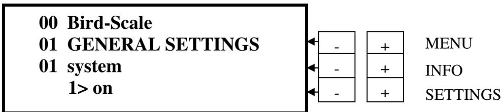
When the Sentinel Scale is installed and first turned on, it will look like this. By pressing the **SETTINGS** “- or +” button will turn the system off or on. (NOTE: You must press and hold the **SETTINGS** “-” button for about 6 seconds to turn the scale off)
