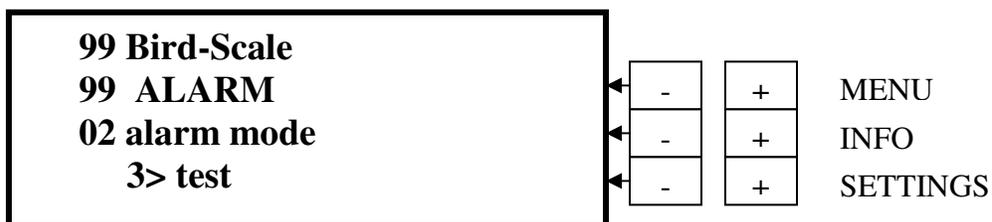
To test the alarm, press **SETTINGS “+”** to get **3> test**. You’ll see the top info **“99 BE-SSC-101 Bird-Scale”** and at the bottom info a **“\*A”**, both will flash on & off. Press **SETTINGS “-”** to go back to **2> on**
