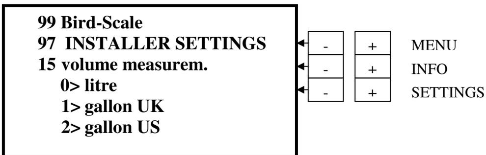
Press **INFO “+”** to go to **info 15**. This is preset to **Litre**. To change the volume measurement from litres to **gallon UK** press **SETTINGS “+”**. To change to **Gallon US** press **SETTINGS “+”** once more.
