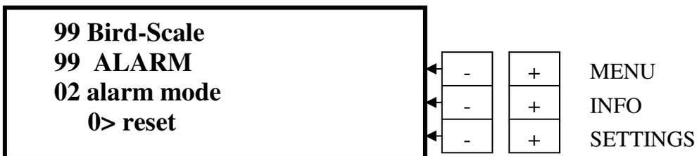
Possible causes of an alarm could mean that there were no weighings on the scales after 24 hours or the house was not turned off after the birds were shipped.
