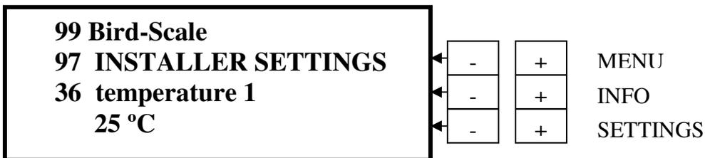
Press **INFO “+”** to go to **info 36**. If the temperature sensor is connected, the actual temperature will show in either **Celsius** or **Fahrenheit** according to what you’ve input previously. If it shows +100 °C or +212 °F, then the sensors are not connected properly. Check the wire connections.
