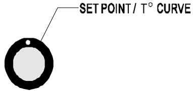
Press the push-button. The word **OFF** is displayed indicating that the temperature curve is deactivated. If this is not the case, see below to deactivate the curve.
