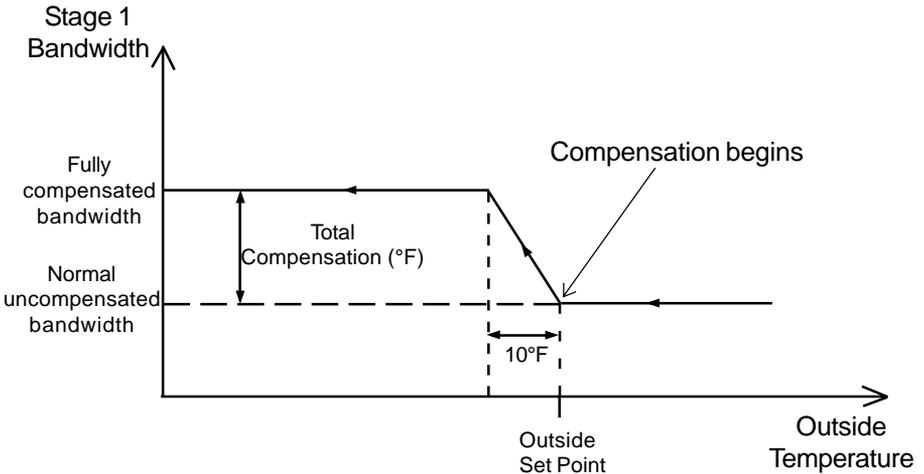
When compensation is in effect, the user can view the level of compensation by placing the selector knob at **STAGE 1 — BANDWIDTH** and waiting 6 seconds: the compensated bandwidth is displayed, alternating with the letters "Ou.C". If no compensation is in effect, no compensated value is displayed.
