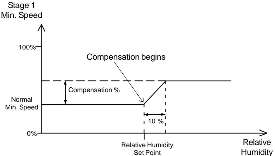
If the minimum ventilation speed curve is activated for Stage 1 fans, the compensation applies to the current minimum speed calculated using the curve. Humidity compensation also applies to the Stage 2 minimum speed if minimum ventilation has been activated. Note that for the compensation
