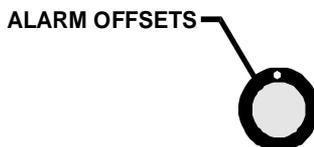
Use the adjustment knob to set the low alarm offset to the desired value.
