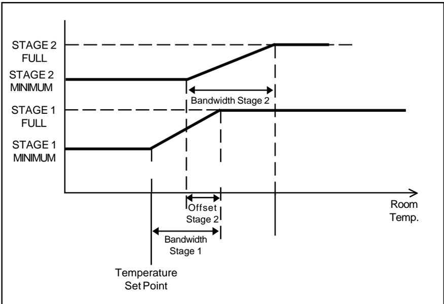
**Figure 3: Operation of Stages 1 and 2 With Negative Offset**
