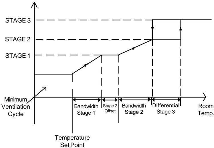
Figure 1: Cooling Operation
