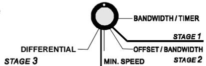
Use the adjustment knob to adjust the bandwidth to the desired value.
