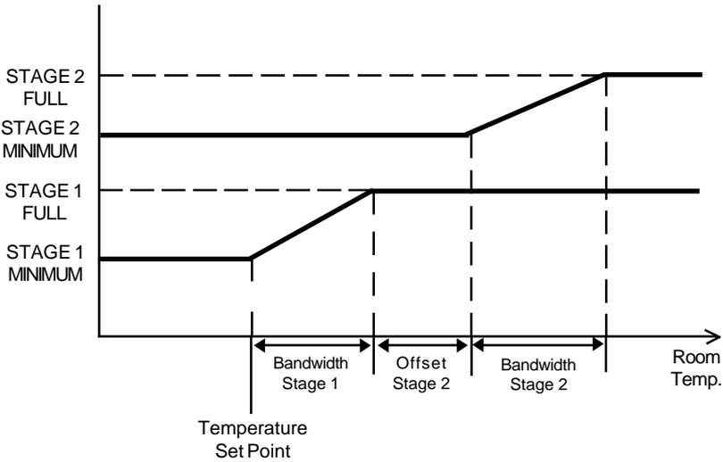
**Figure 2: Stage 1 and 2 Operation showing Minimum Ventilation**
