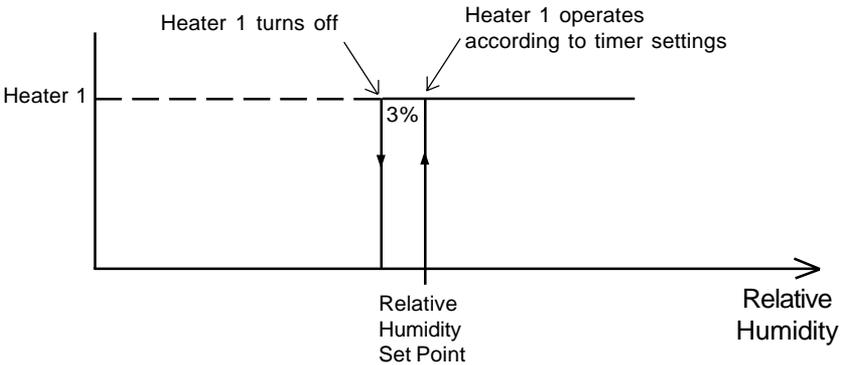
Heater 1 operates according to timer settings as shown below:
