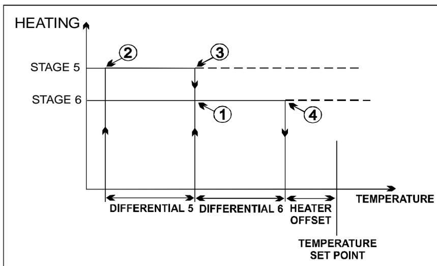
When stages 5 and 6 are used for heating, stages 1, 2, 3 and 4 operate as described for cooling. However stages 5 and 6 operate at room temperatures below the set point, as described hereafter.
