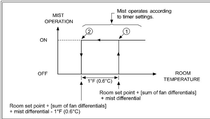
Time on [minutes] - The mist units operate according to a timer cycle. The time on is the running time of the mist units.
