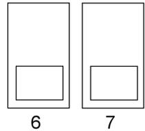
**FACTORY SETTING:** When the controller is shipped from the factory, switch #6 is set to OFF and switch #7 is set to OFF (stage 5 and 6 used for cooling).
