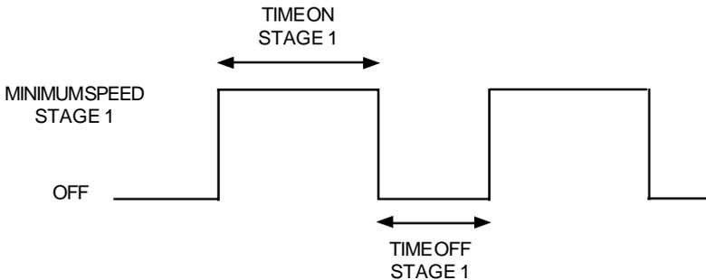
Time on [seconds] - When the stage 1 fans operate according to the minimum ventilation cycle, they run during time on.
