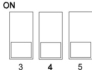
**FACTORY SETTING:** When the controller is shipped from the factory, switches # 3, 4 and 5 are set to OFF (probes are deactivated).
