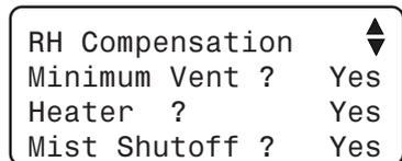
**Heater Timer:** Press the Edit key and set to Yes to use the heaters in timer mode in order to decrease the humidity level when it is too high.
