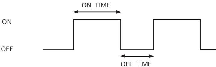
When the cooling cycle starts (**On Temp**), the output is activated using the **minimum ON time** that has been defined by the user. The ON time gradually increases as the room temperature increases. The **maximum ON time** is reached when the room temperature reaches the Max Temperature value (**T° Max**), this value is also defined by the user. The OFF time in a cooling cycle always remains the same. The following graphic illustrates the situation:
