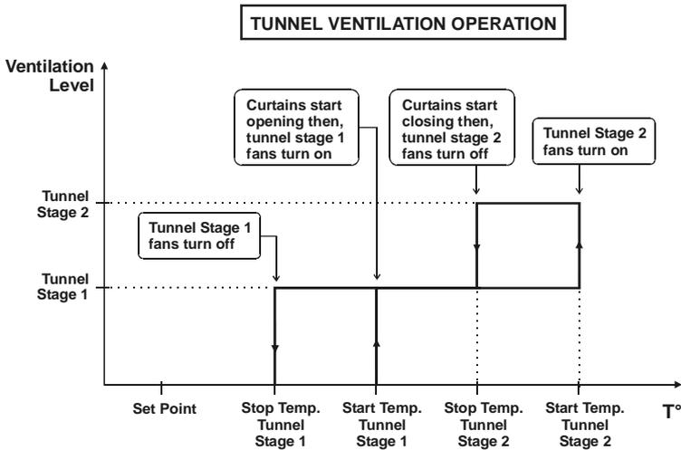
A minimum animal age is defined to avoid starting the tunnel ventilation when the animals are too young. The user must also define a minimum outside temperature: the tunnel ventilation is never activated unless the outside temperature is sufficiently warm.
