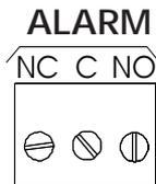
There are two types of alarms on the market. One type activates when current is cut off at its input, whereas the other activates when current is supplied at its input. For an alarm of the first type, use the NC terminal as shown on the wiring diagram. For an alarm of the second type, use the NO terminal.
