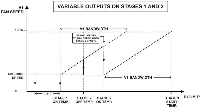
If the last fan stage uses variable outputs, it must be configured in ON-OFF mode (see sec. 5.16.7.2).
