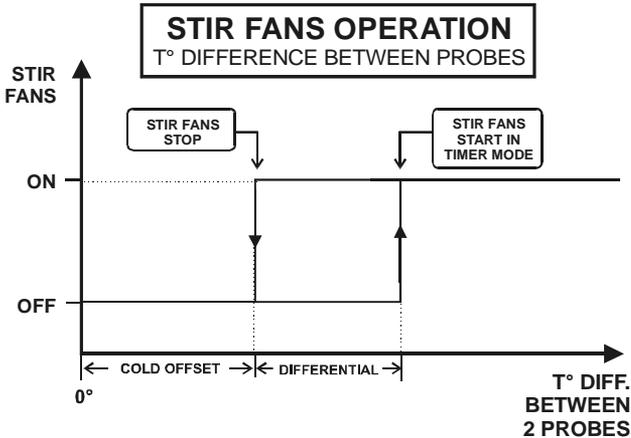
If the temperature difference between two active probes exceeds the cold offset + the stir fan differential, the stir fans are turned on. When the temperature difference returns to a value less than or equal to the cold offset, the stir fans are turned off.
