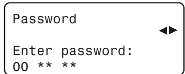
The second two-digit number flashes on the display. Press the Edit then use the up and down-arrow keys to set the second number. Proceed in similar fashion to set the third two-digit number. Press the right-arrow key one last time to validate the complete password.
