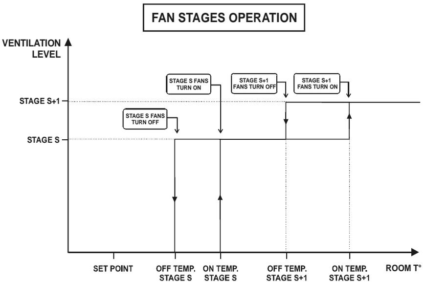
Start temperatures (ON TEMPS) are defined with respect to the set point and with respect to each other. This means that when one of these values is adjusted, all the consecutive values are adjusted by the same amount. For example, if the set point is increased by 1° F, the start temperatures for all fan stages will be increased by the same amount.
