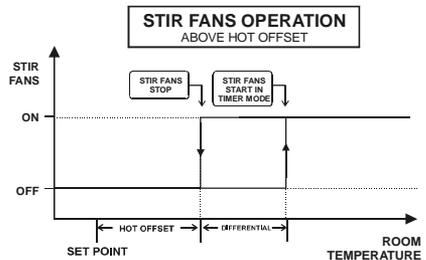
The controller also offers the possibility to mix the air if the temperature DIFFERENCE BETWEEN TWO PROBES is too high. The following graphic illustrates this.
