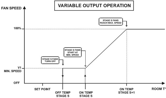
If the next stage is an ON/OFF fan stage, the variable output is deactivated when the new stage starts. If the next stage is another VARIABLE fan stage, the speed of the first variable stage is reduced to its minimum speed when the second variable stage starts. The graphic below illustrates this situation.
