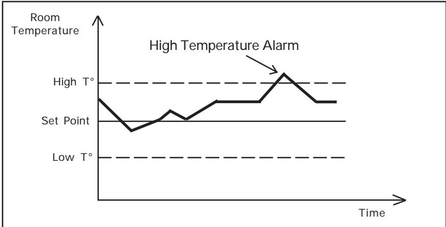
When the average room temperature exceeds the high temperature alarm setting, a high temperature alarm is generated. When the average room temperature drops below the low temperature alarm setting, a low temperature alarm is generated. Although these settings are entered by the user as absolute values, they are defined relative to the current set point and are automatically adjusted by the controller when the set point changes.
