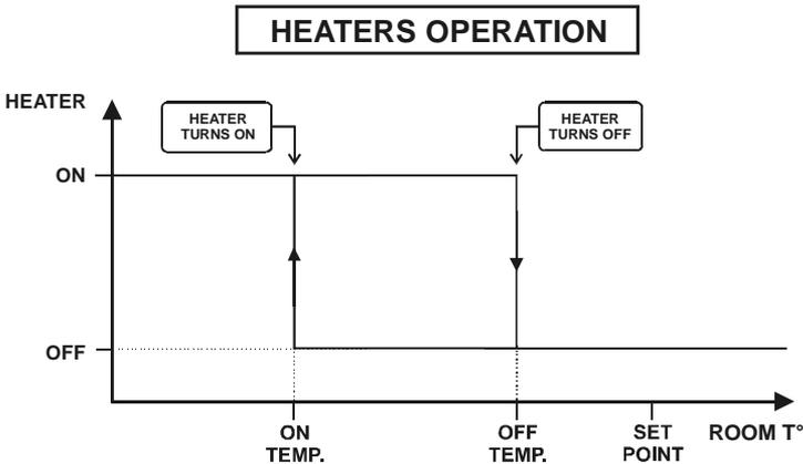
The stop temperature of an heater stage must be at least 0.5° F (0.3° C) higher than its start temperature. The start (On) temperature can be set from 0.5° F (0.3° F) below the set point to -40° F (-40° C). The number of heater stages and their probe assignment are defined during the installation (see sec.5.16.3 and 5.16.4).
