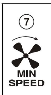
When room temperature is at the Fan 2 relative set point, Fan 2 runs at minimum speed set by this function. This value is entered as a percentage of fan maximum speed. The Fan 2 minimum speed is adjusted in 2% increments from a minimum setting of 12% to a maximum setting of 100%.
