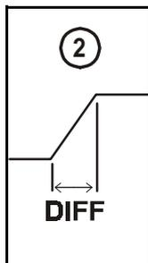
The Fan 1 differential is adjusted in 0.5 degree increments from a minimum setting of 2.0° F (1.0° C) to a maximum setting of 18.0° F (10.0° C).
