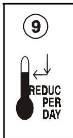
The reduction setting is adjusted in 0.01 degree decrements from a minimum setting of OFF,  $-0.01^{\circ}\text{C}$  ( $-0.01^{\circ}\text{F}$ ) to a maximum setting of  $-0.50^{\circ}\text{C}$  ( $-0.99^{\circ}\text{F}$ ).
