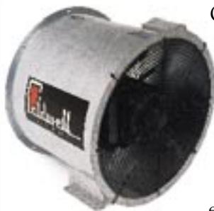
Caldwell axial fans operate at 3450 rpm to deliver maximum air performance in low static pressure applications. Diameters range from 12" to 28", with horsepower ranging from .75 to 12.5. Fan housings are constructed of heavy gauge galvanized steel and equipped with safety screens to meet OSHA standards.
