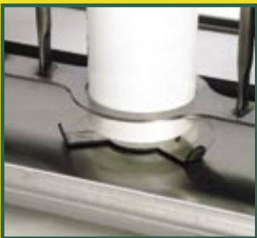
Spinner agitator keeps feed from bridging.
