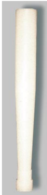
Drop tube is 27" long with 3-1/16" ID inlet for easy attachment to the feed drop. Outlet end of drop tube has 2", 2-1/16", and 2-3/8" ID steps for easy attachment to your stall.
